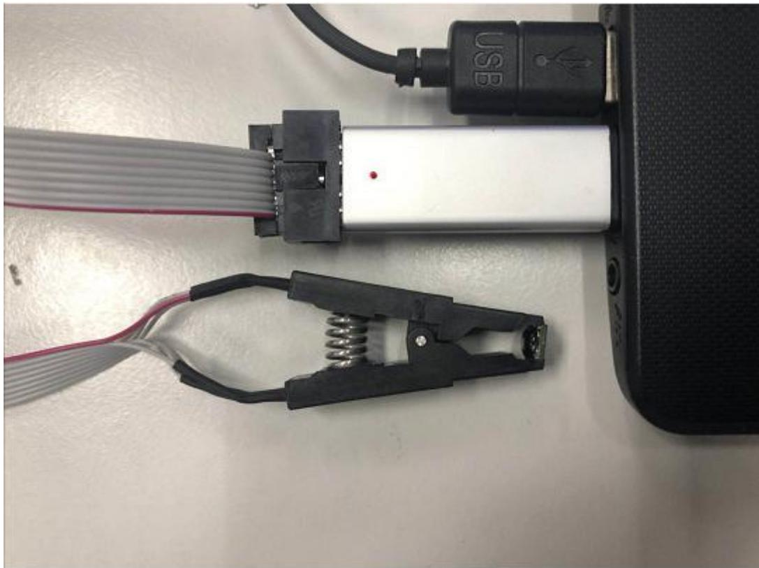
8. Select EEPROM model, click "Load Data File", Select the corresponding data of original EEPROM and load it. Check whether the displayed mileage is the same as the mileage displayed in odometer.
